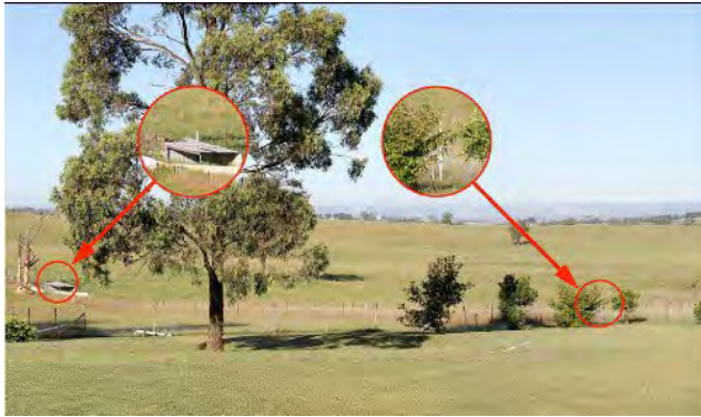
Physical 3000mm site poles placed at lot corners 3d poles located in the 3d model and positioned on photo
